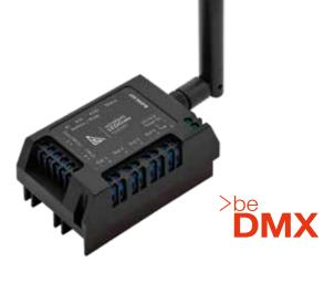
LEDGate NANO is compact LED driver with DMX512 (DMX512/RS-485 for wireless) inputs. Powered from 12/24 VDC source, LEDGate is capable to control and dim 2 or 4 output lines for direct connection with LED equipment: duralight, driverless LED luminaires, etc, with independent short-circuit protection on each
