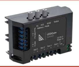
The LEDGate Slave Nano expands the channel capacity of LEDGate Nano, Wireless Nano, and Bare devices, serving as a configurable power supply for DMX512-controlled LEDs. It manages four PWM LED channels with short-circuit protection, precise dimming, flicker-free operation, and 8/16-bit control. Powered by 12-24V DC, it supports RDM (ANSI E1.20) and rotary switch configuration. Its compact, lightweight design allows versatile placement on stage elements, sets, and various surfaces.
